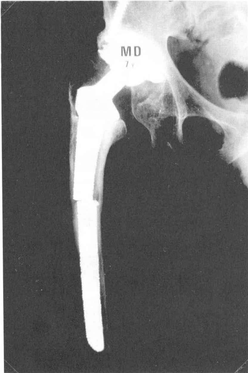
Figure 7.12. Stress corrosion cracking on a hip prosthesis of stainless steel.
